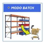
The proposed solution is to use a trolley with a Tablet and a scanner. The operator performs a grouped collection of items by the warehouse and then can be sorted on a shelf SORTER.
