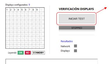
It is a tool that allows us to check the installation map of the displays, identifying with green color those that are connected and in red those that are missing.
