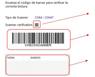
If this green "Scanner verification" led is not activated, it will not be possible to work in any Picking, Trolley, etc. mode.
